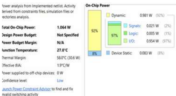
Fig 6. Power report of Johnson counter with clock gating
