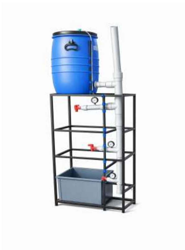
Figure 1. Water Pressure System
