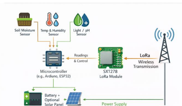
Figure 2: System Architecture of Receiver unit
