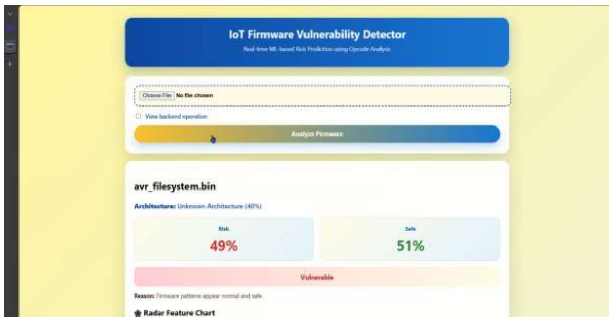
Fig. 2. Output of Firmware Vulnerability Detection System
