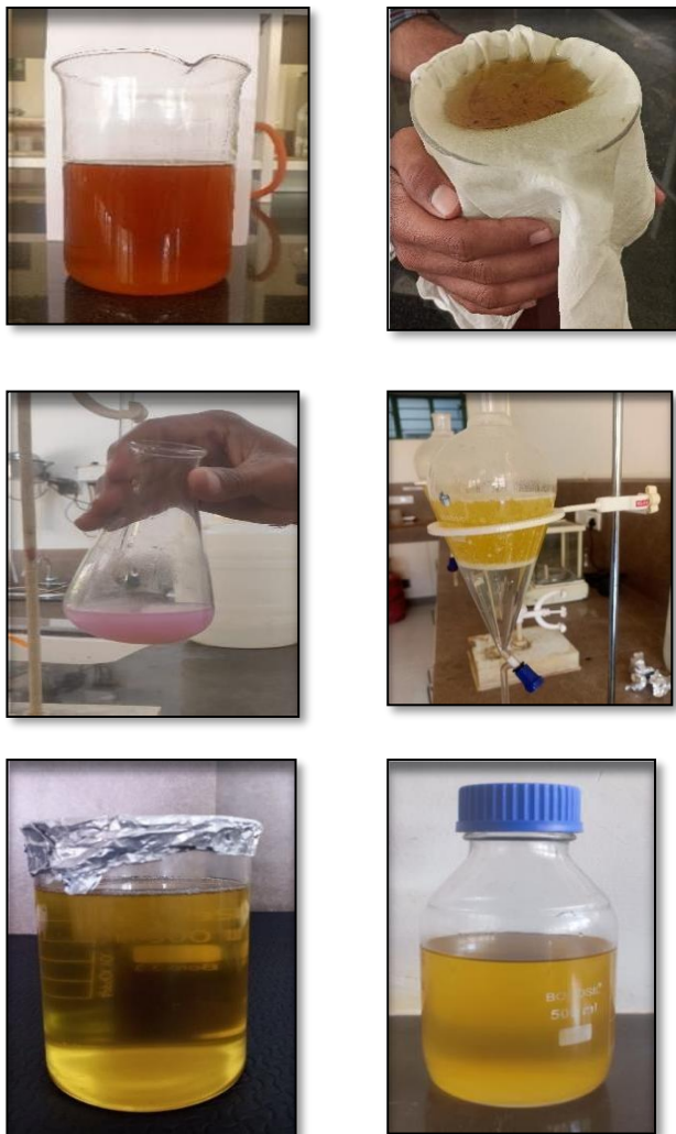
Figure 2. Visual workflow of Biodiesel production using UCO
