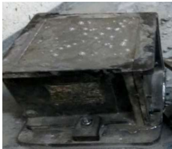
Figure 5.9 Air Bubbles Travelling to the Top of the Surface
