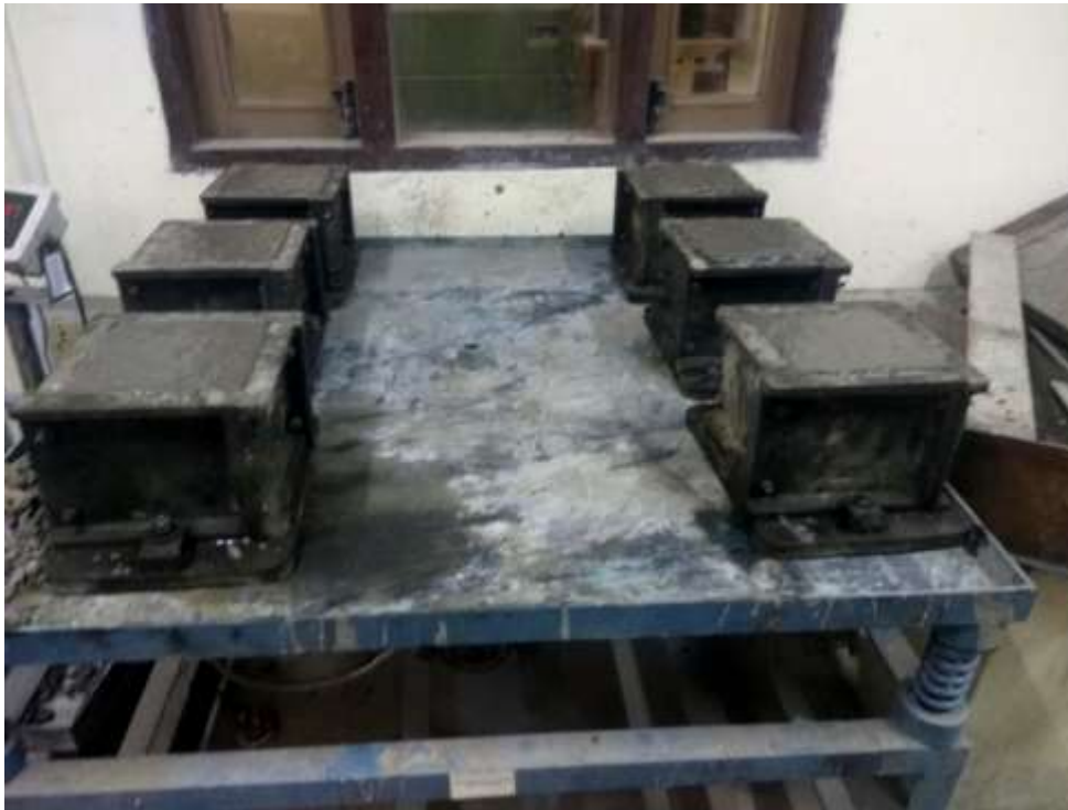
Figure 5.8: Table Vibrator to Emit out Entrapped Air
