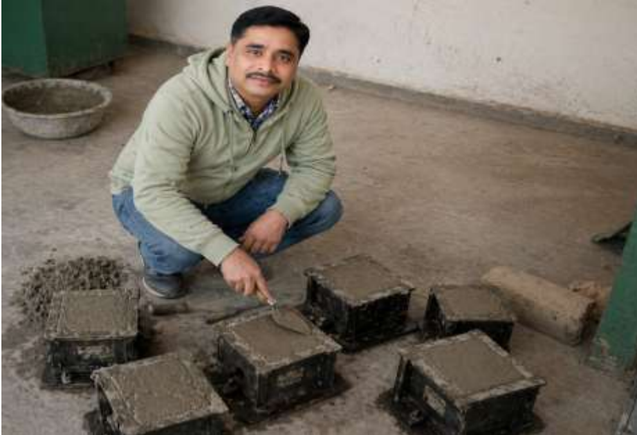
Figure 5.7: Levelling and Finishing of Top Surface
