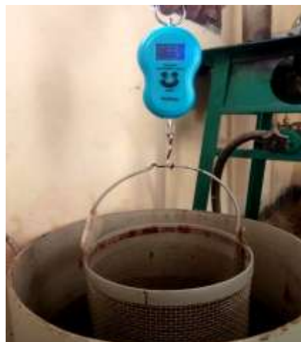
Figure 4.1: Weight of Aggregate Along With Wired Basket Immersed in Water Filled Bucket
