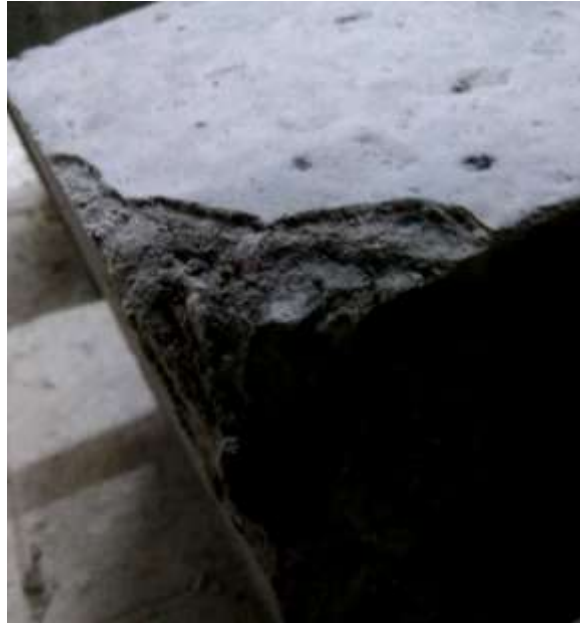
Figure 5.10: Broken Edge of Cube Demoulded Without Rest Period
