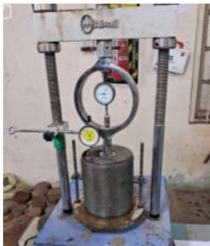
Fig 7: CBR Test Setup for Stabilized Soil Sample
