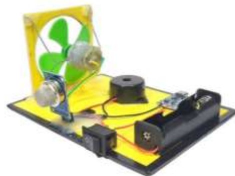
Fig. 1 Gas Leakage Detection with Automatic Exhaust Fan
