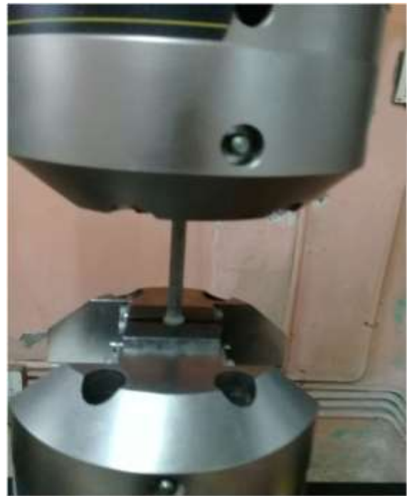
Fig.3 (a) Fatigue Testing machine Instron 8801 (b) Specimen inserted between the hydraulic-controlled jaws.
