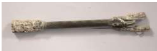
Fig.4 Fracture modes of sand-coated BFRP specimen
