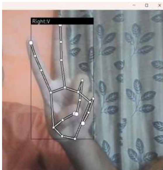
Figure 2: Real-time hand detection, landmark tracking, and gesture classification output (Letter 'V')
