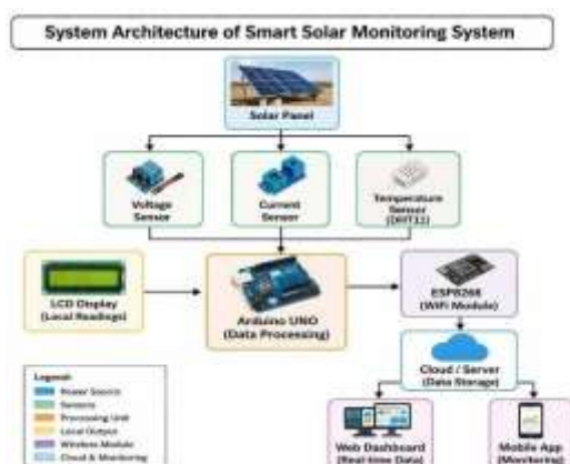
Fig 2 : Workflow of Smart Solar Power Monitoring System Architecture
