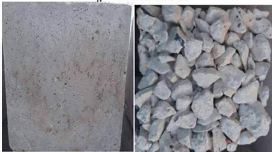
Fig 1.2 Comparison of Normal Concrete and Pervious Concrete
