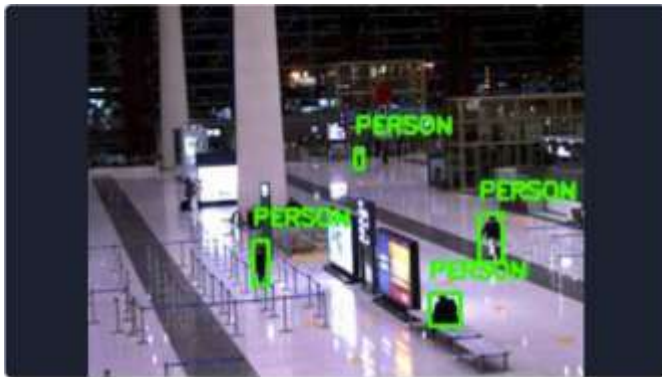
Fig. 2. Output frame from the YOLOv8 perception stage, showing detected bounding boxes.
