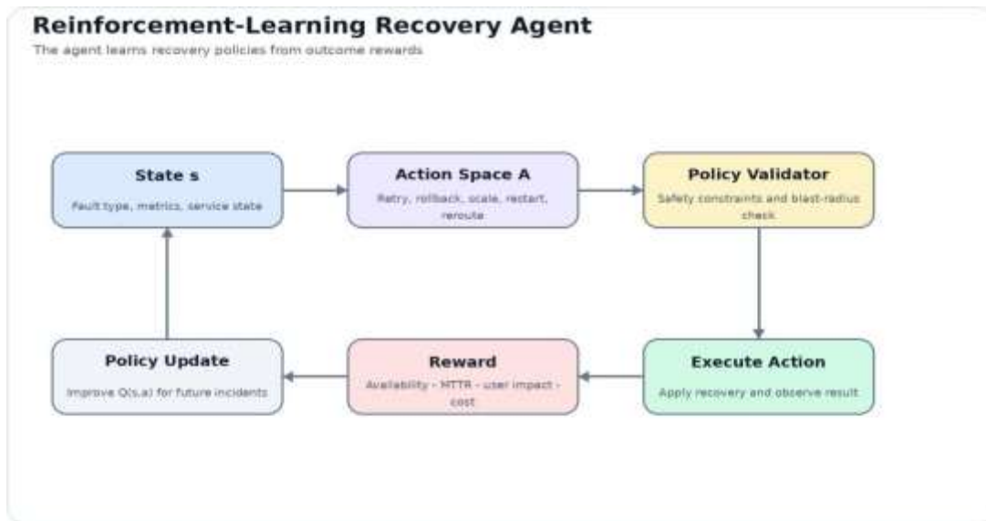
Fig. 7. Reinforcement-learning recovery agent with policy validation and reward feedback.
