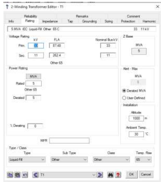
Fig.4.4. Ratings of Transformer (33/11 kV)
