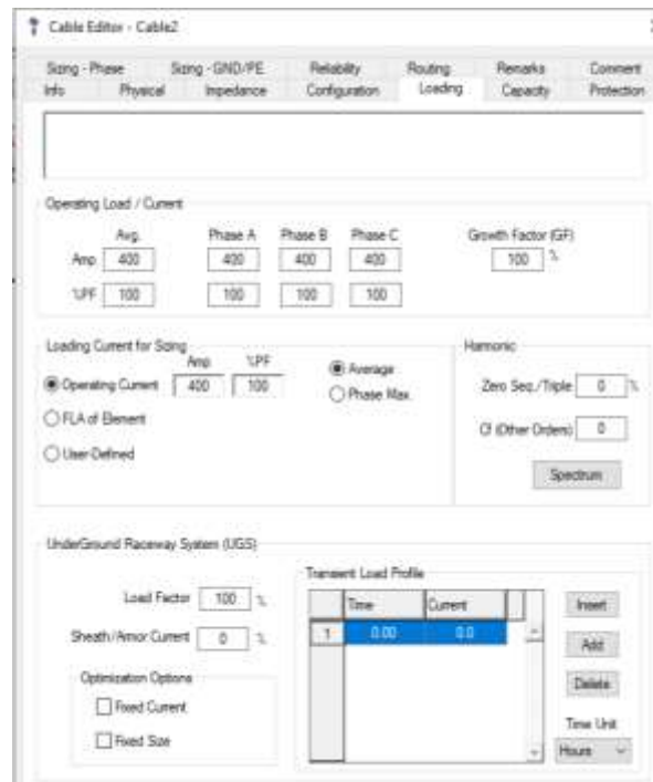
Fig.4.7. Operating Current capacity of cable
