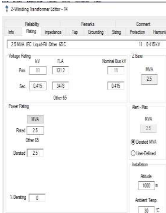
Fig.4.8. Ratings of Transformer (11/415 kV)
