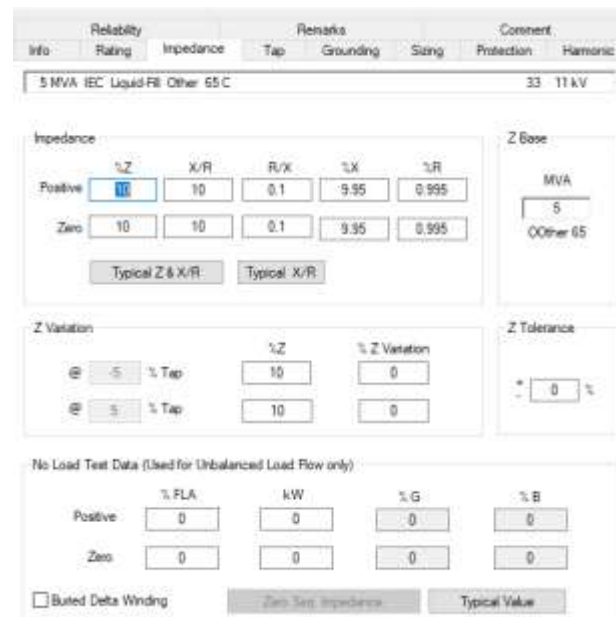
Fig.4.5. Transformer (33/11 kV) Impedance Ratio
