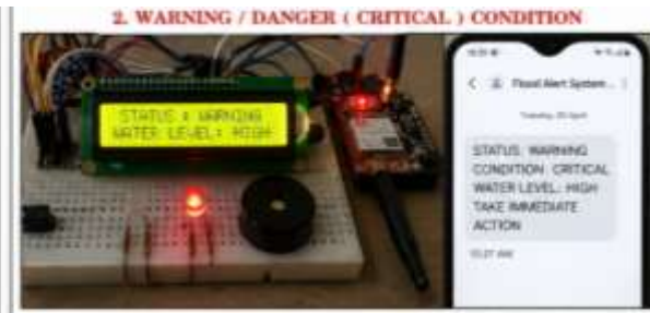
Fig 9.2 Warning / Danger (Critical) condition – Red LED ON, LCD display and SMS alert
