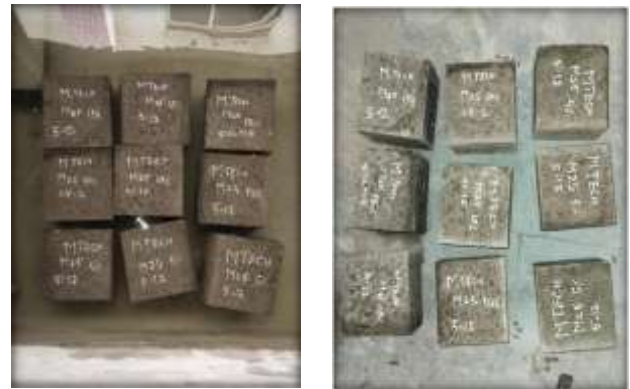
Fig.1. Casting of cubes for trial mix (a), curing of trial mix cubes(b)
