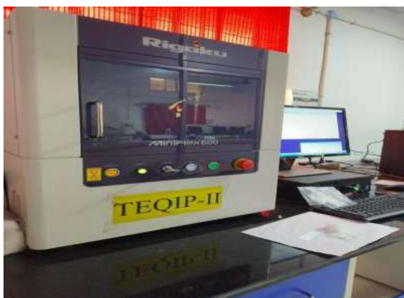
Figure 5.1 Experimental setup of X-ray diffraction analysis
