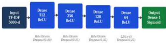
Fig. 5. SpamShield DNN architecture. Input dimensionality is 5,000. BatchNorm and progressive Dropout after each hidden layer regularise the model.
