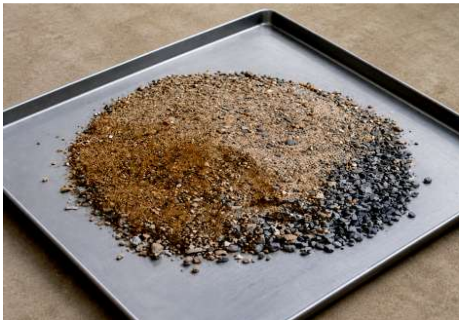
Figure 4.1 Dry Mixing Materials
