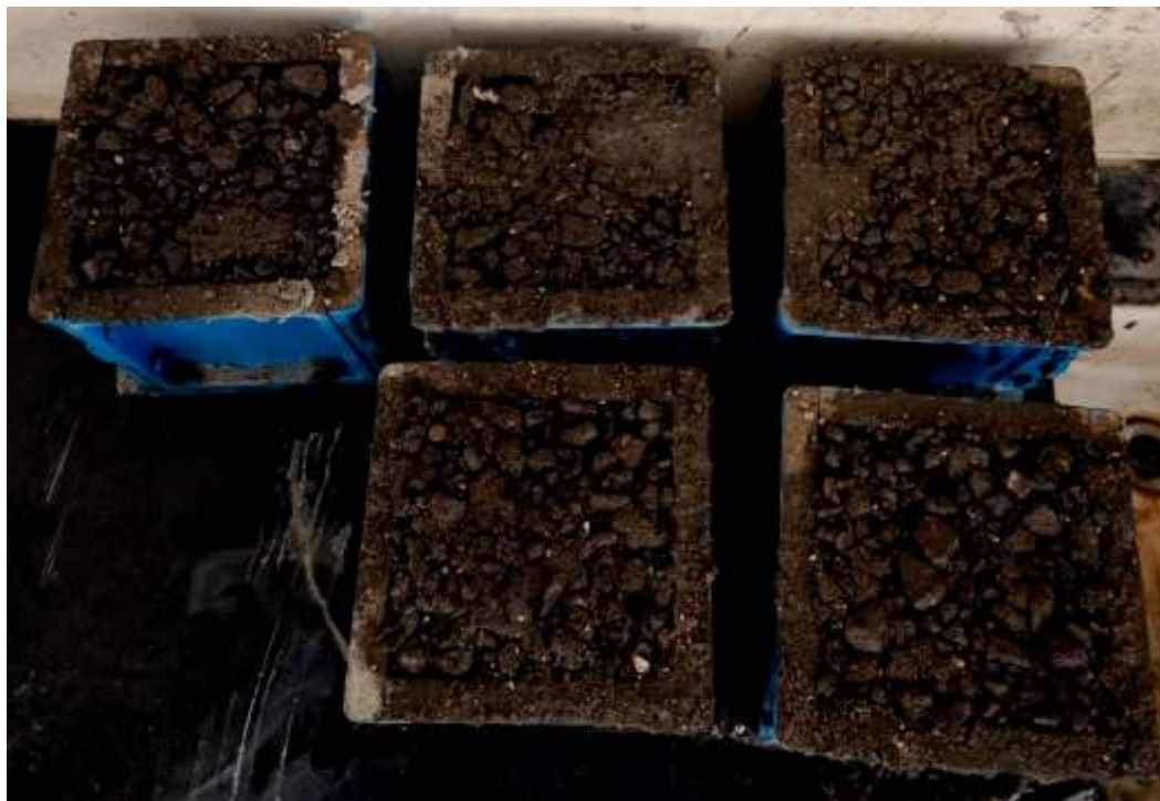
Figure 4.3 Cube Casting With Mould
