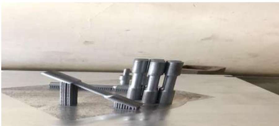
Figure 1 Build orientations of SLM-fabricated AlSi10Mg tensile specimens.
