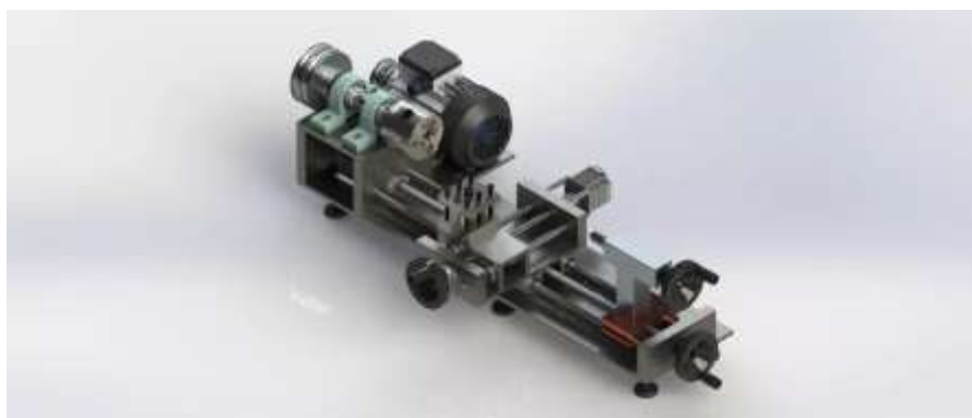
Figure 1. 3D CAD Model of the Proposed Mini Lathe Machine
