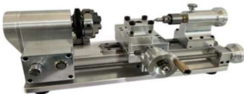
Figure 3. Fabricated Prototype of the Mini Lathe Machine
