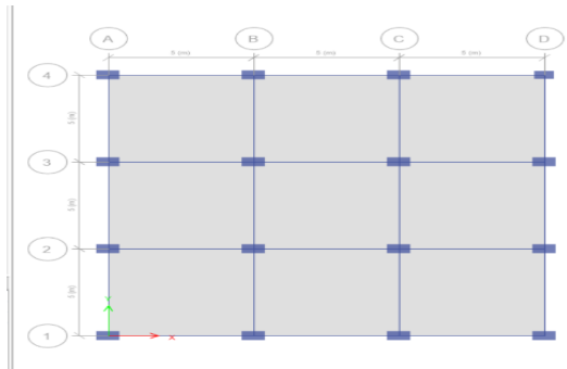
Fig. 2. Ground Floor Plan Layout (4×4 grid, 5 m bay spacing)
