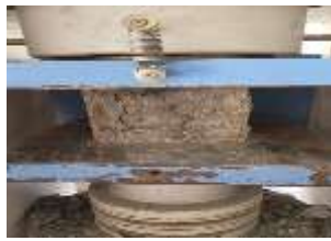
Fig. 2: Typical failure pattern of cube specimens under uniaxial compression
