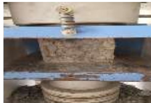
Fig. 3: Post-failure appearance of high-strength M60 FAP cube specimen
