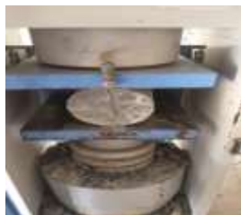
Fig. 4: Cylinder specimens undergoing split tensile testing typical diametral splitting failure
