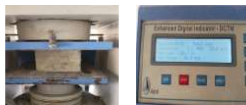
Fig. 4.2: (a) Cube specimen positioned in Aimil DCTM prior to testing;
