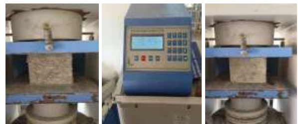
Fig. 4.1: Representative DCTM readings Record No. 01250 (76.38 MPa, M60 NC/56d), 01253 (35.69 MPa), 01263 (60.74 MPa)
