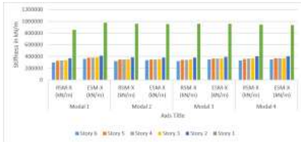
Fig.17 Comparison of Storey stiffness of all storeys in X direction by RSM and ESM with all models
