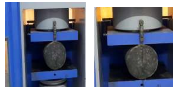
Fig-9: Split Tensile Strength test set-up / Specimen
