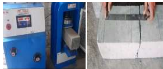
Fig-8: Flexural Strength test set-up / Specimen
