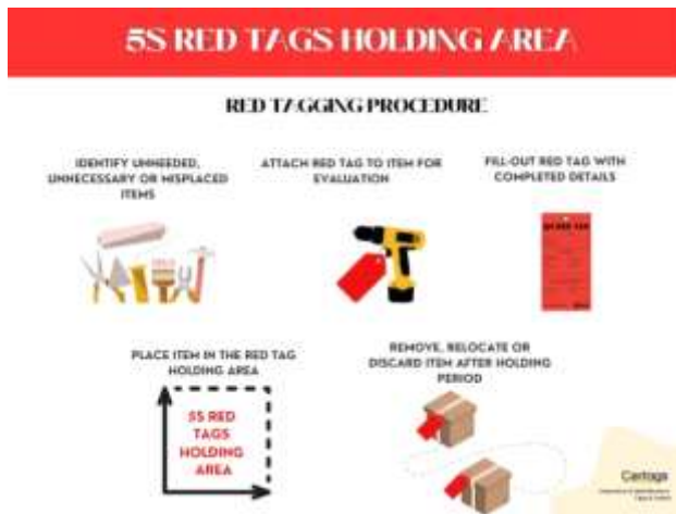
Figure 3. Red tag system used to identify unnecessary materials during the Sort phase.
