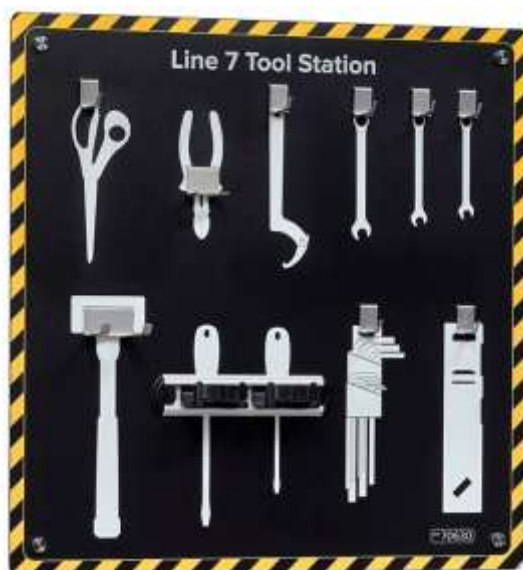
Figure 4. Shadow board used for organized storage and quick identification of tools.
