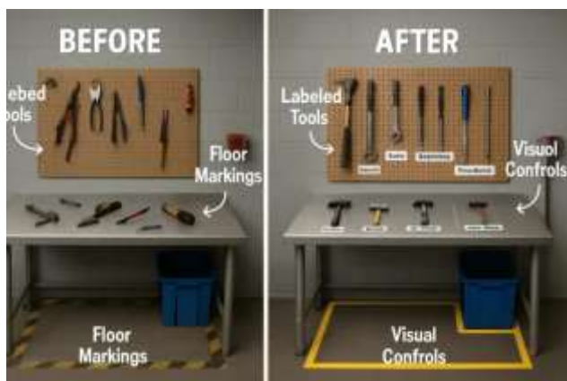
Figure 2. Comparison of a manufacturing workstation before and after implementing 5S practices.
