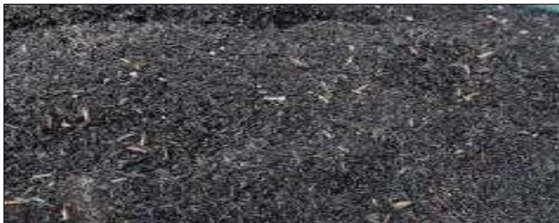
Figure: Ricehuskwasconvertedintoashbyopenburningmethodatatemperature rangingfrom300°Cto450°C(Stage-II)
