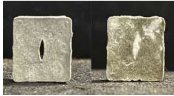
Fig.2: cube casted with self-healing material
