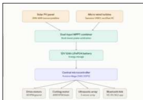
Figure 1. Block diagram of the proposed hybrid solar-wind powered autonomous grass-cutting machine, showing power flow from the solar PV panel and micro-wind turbine through the dual-input MPPT combiner to the LiFePO4
