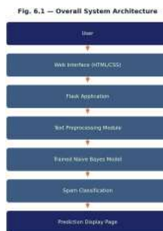
Fig. 6.1. Overall system architecture.
