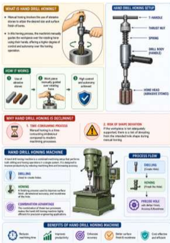
Figure. 11 Working of Drill Honing Machine
