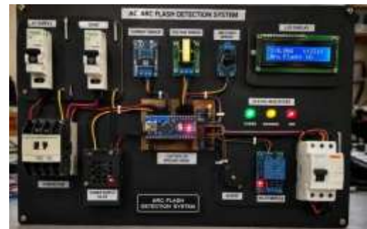
Fig. 4. Hardware prototype of the AC arc flash detection and protection system.
