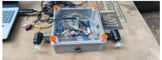
Fig. 2. Assembled ROV showing the two horizontal thrusters and front-mounted camera.
