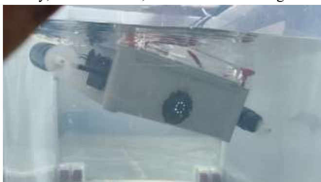
Fig. 3. Underwater testing of the developed ROV in a controlled water tank.
