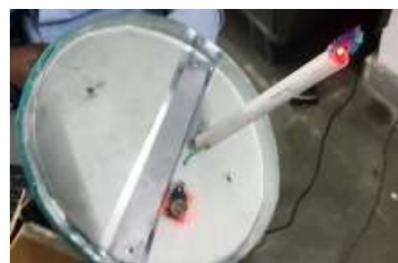
Fig. 3. MQ-135 gas sensor mounted on the storage container lid.
