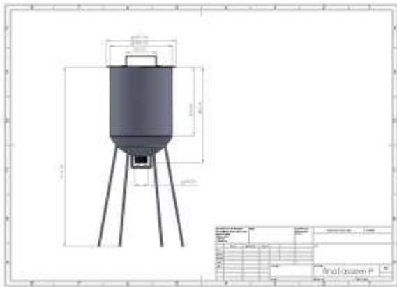
Fig. 4. CAD assembly drawing of the grain storage container (dimensions in mm).
