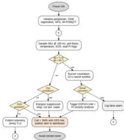
Fig. 2. Main control flowchart of the ESP32 firmware. Connector A return to the sensing loop.
