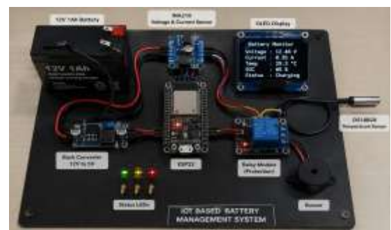
Fig. 1. Assembled IoT-based BMS hardware prototype.
