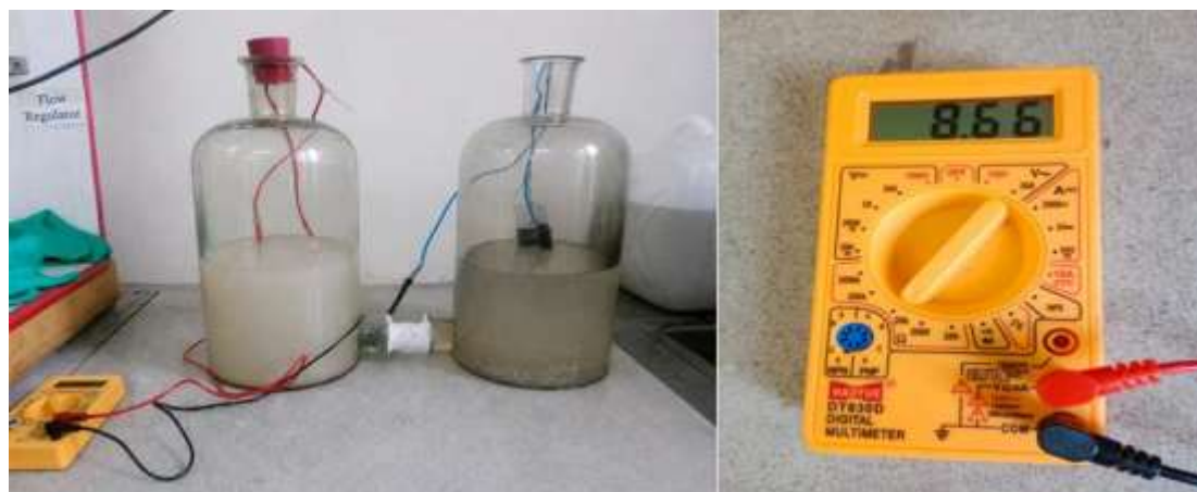
Fig 7: Voltage Output of MFC System
