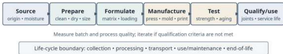
Fig. 1. Review-derived pathway from residue sourcing to component qualification; life-cycle inventory spans the full value chain [13], [14], [17].
