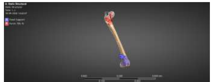
Fig. 5. Boundary conditions for the fractured femur with Implant 1: fixed support (A) at the distal end and 700 N force (B) at the proximal end.
