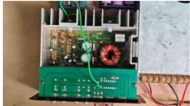
Fig. 2. Class-D amplifier/power stage used in the prototype
