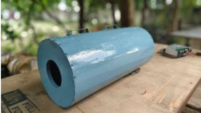
Fig. 4. Fabricated directional acoustic enclosure
