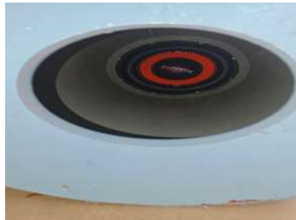
Fig. 3. Horn-loaded low-frequency driver used in the prototype
