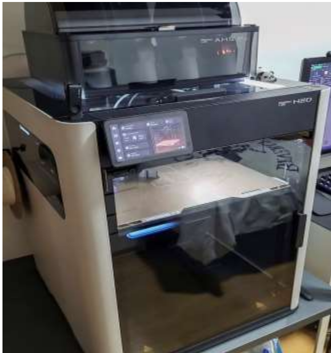
Figure:5 'Dual-gear direct-drive Bambu Lab P2S and H2D additive manufacturing platforms.
