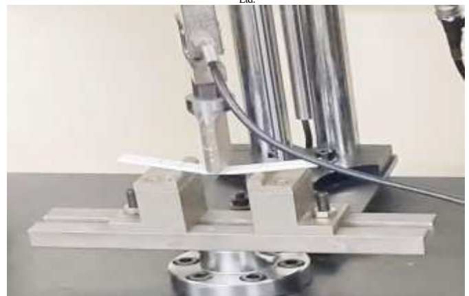
Figure:7 Clamping fixtures for ASTM D638 tensile testing and ASTM D790 three-point flexural testing.
