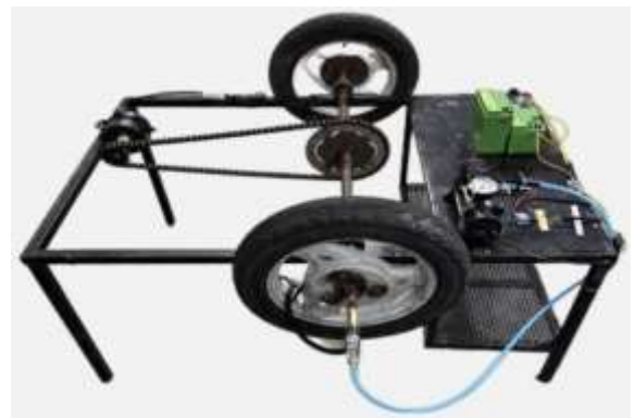
Fig. 2. Fabricated prototype of the automated tyre inflator and deflator system.
