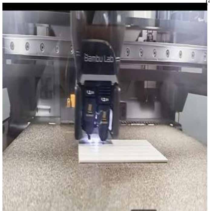
Fig. 3. In-situ deposition of prismatic flexural coupons on the heated bed
