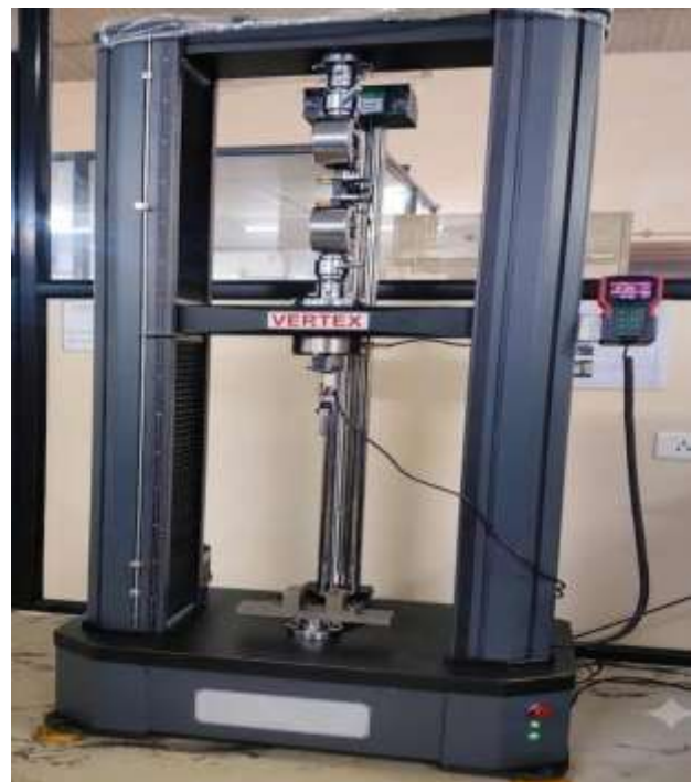
Fig. 6. VERTEX 50 kN Universal Testing Machine setup during flexural testing.
