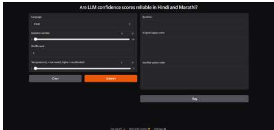
Figure 3. The demonstration app on start-up. The controls on the left set the language, question number, shuffle seed and temperature; the question and the original and shuffled option orders appear on the right.
