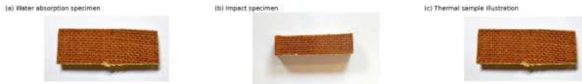
Fig. 4. Specimens prepared for water absorption, impact and thermal characterization.
