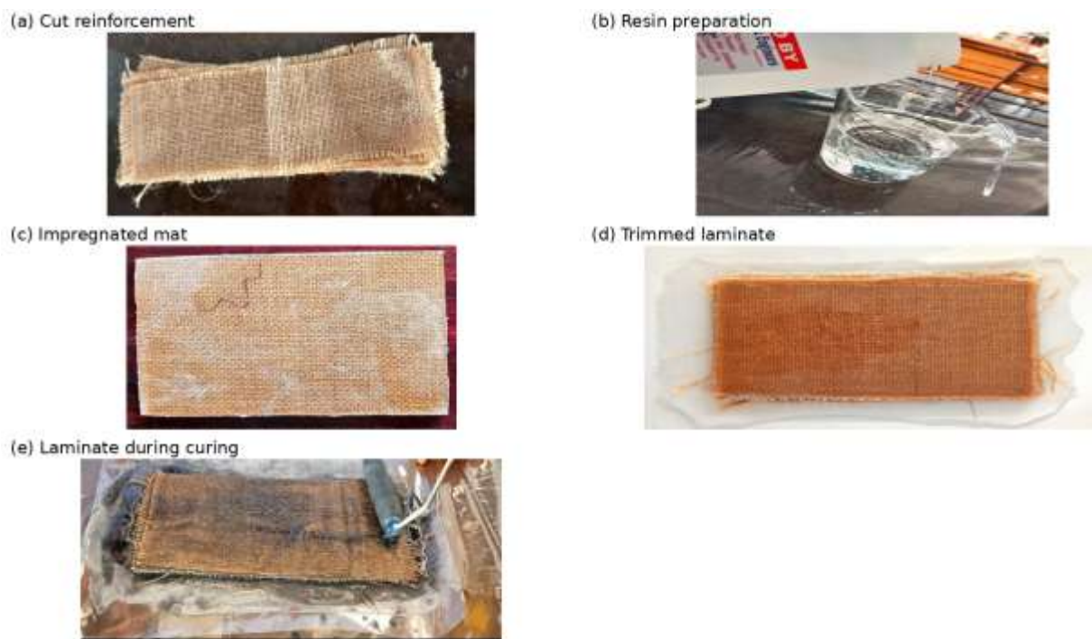
Fig. 2. Major stages involved in the fabrication of the jute–epoxy composite laminate.
