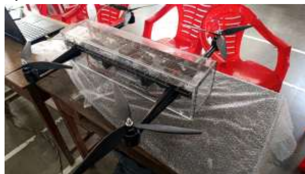
Fig. 2. Preliminary prototype assembly showing the central body, supports and rotor units.
